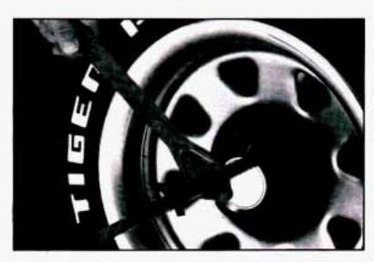
Place the ratchet and socket end of the extention on the wheel nut with the center cap on.
